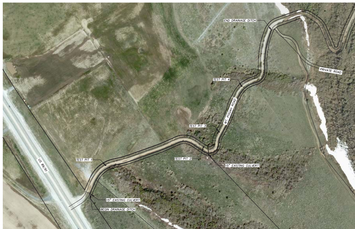
MT. PISGAH ROAD DRAINAGE PLAN SCALE: 1" = 150'
